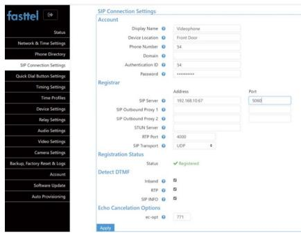
Screen name: enter a logical name for the device. The device's location is useful when you have multiple door intercoms in 1 project.
